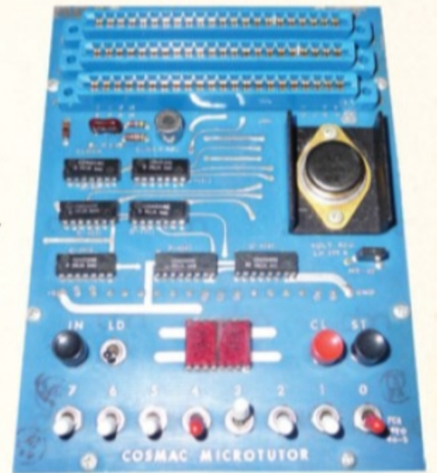
» An impressive closeup of the COSMAC Microtutor main unit. The main processing parts are on removable cards that dock in the empty slots shown.
